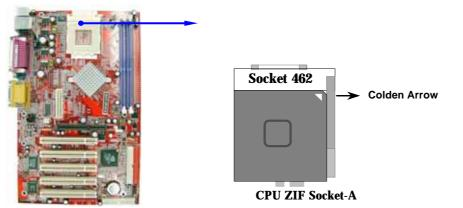
When you insert the CPU onto the ZIF socket, no force is required. After inserting, press the lever slightly without any extra force to lock CPU in position.
